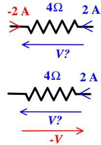
The solution to the example above includes negative values of voltage and current. Negative values of variables will occur routinely during the analysis of circuits and need not cause any concern, as illustrated in the following examples.
