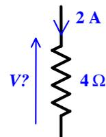
Ohm's Law can be applied only when the voltage and current directions are as defined in Fig. 1.3, in which both the voltage and current arrows point at the same end of the resistance. Before applying Ohm's Law, as in the example above, it is essential to check that the voltage and current directions are defined in a way that is consistent with the Law. If the directions are inconsistent, then the problem needs to be approached carefully, as shown in the following example.
